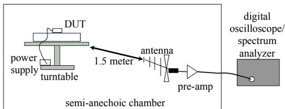
Figure 1. Measurement of emissions in 3-meter chamber.
