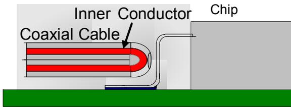
Figure 11. Slotted coaxial cable probe.
