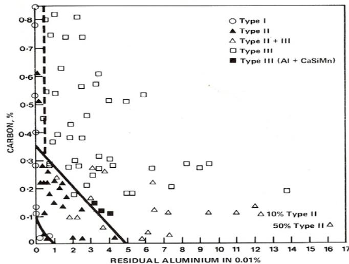
**Figure 5:** Effect of Carbon and Aluminum on Sulfide Shape<sup>8</sup>
