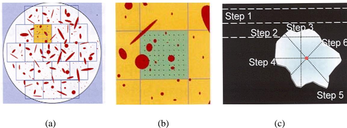
**Figure 7:** Automated inclusion analysis including a) subdividing the image into fields, b) moving electron beam across field in an array and c) sizing and cataloging of particles detected by back scattering electrons and centering the beam on each particle and obtaining composition by x-ray spectroscopy<sup>11</sup>
