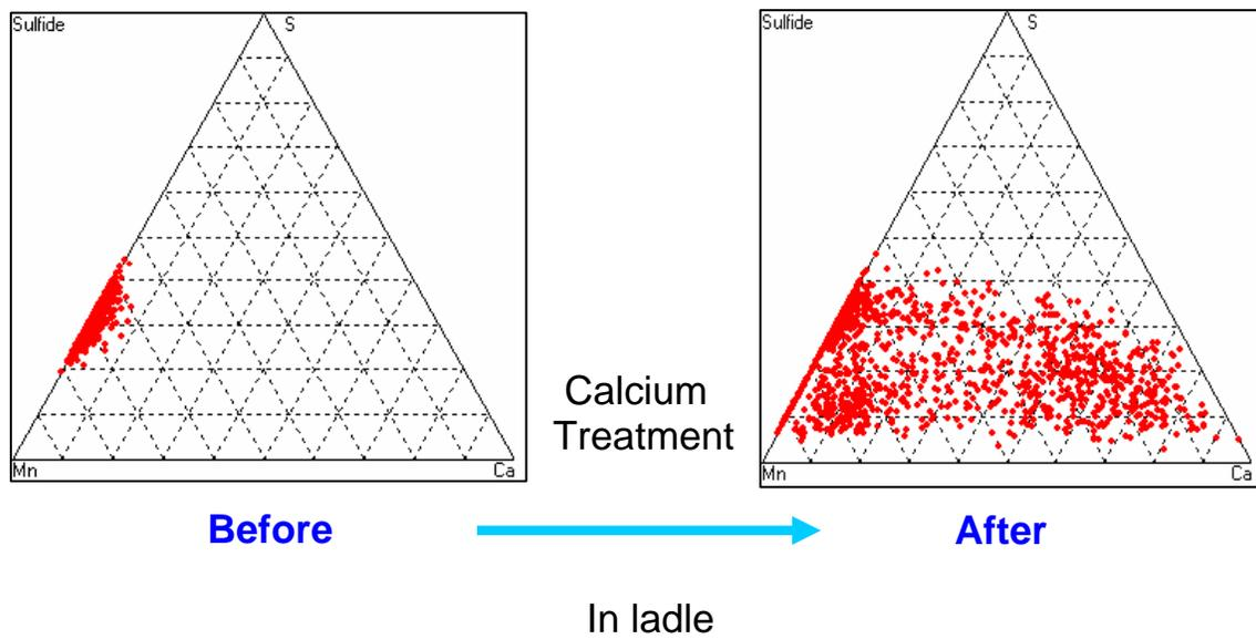
**Figure 12:** Ternary Mn-Ca-S diagram for casting process, before and after addition of Ca in ladle (Plant B).
