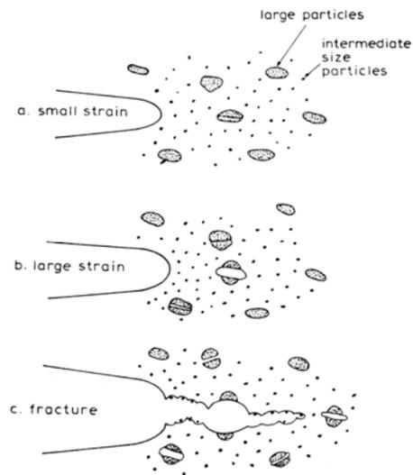
**Figure 1:** Nucleation of voids on primary inclusions (a, b) and fracture of steel (c)<sup>1</sup>
