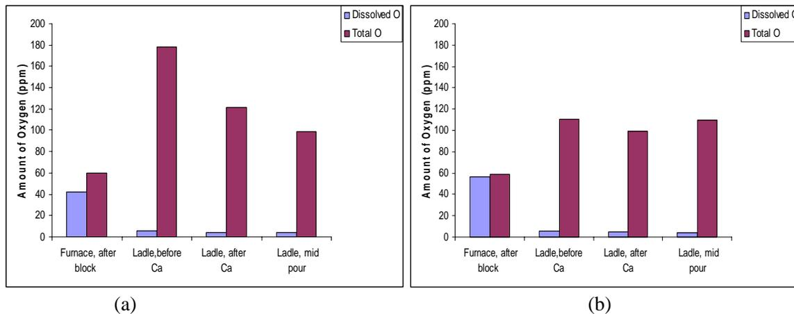
**Figure 15:** Dissolved and total oxygen measured in samples collected at various stages of the casting process for (a) acid and (b) basic process (Plant C).
