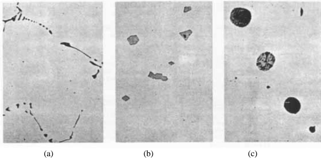
**Figure 6:** Sulfide inclusions (a) Type II, 0.009 % Al residual content after deoxidation (b) Type III, 0.03 % residual Al content (c) Type I, Si-killed (all at 500X).<sup>9</sup>
