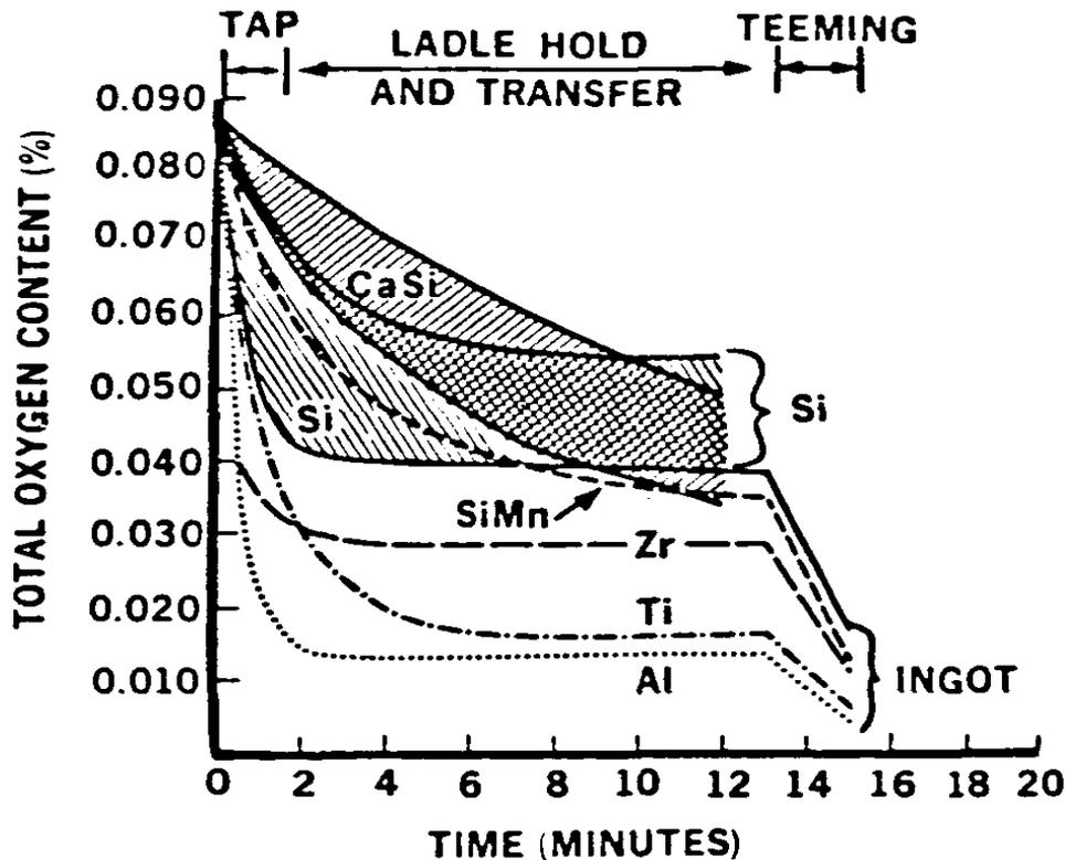
Figure 2: Deoxidation results of the common deoxidizers<sup>3</sup>
