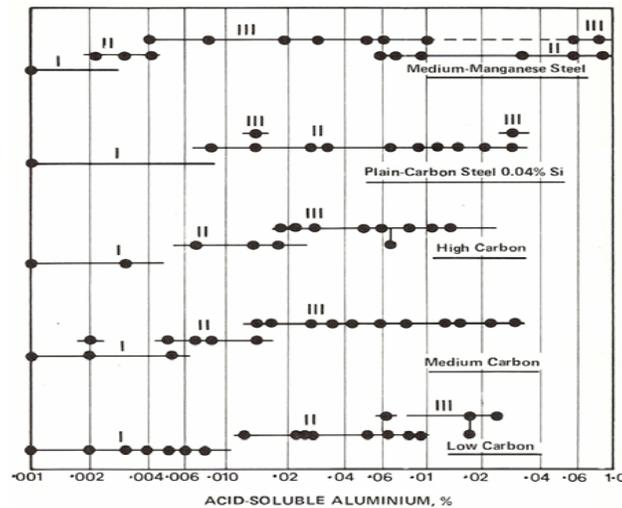
**Figure 4:** Effect of chemistry on sulfide morphology<sup>7</sup>
