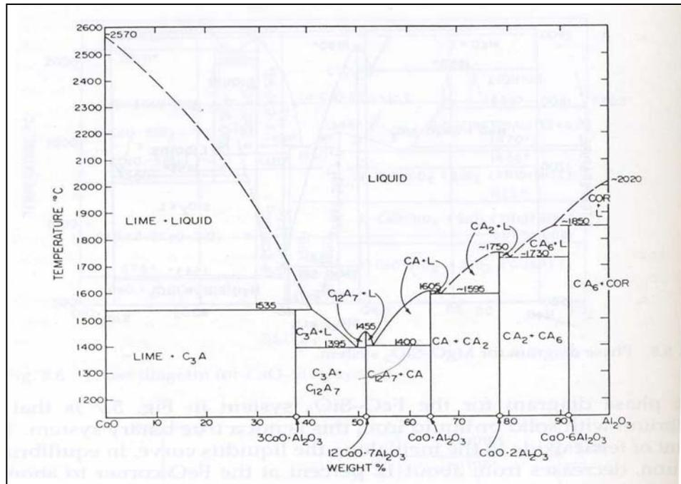
**Figure 3:** CaO- Al<sub>2</sub>O<sub>3</sub> binary phase diagram<sup>5</sup>
