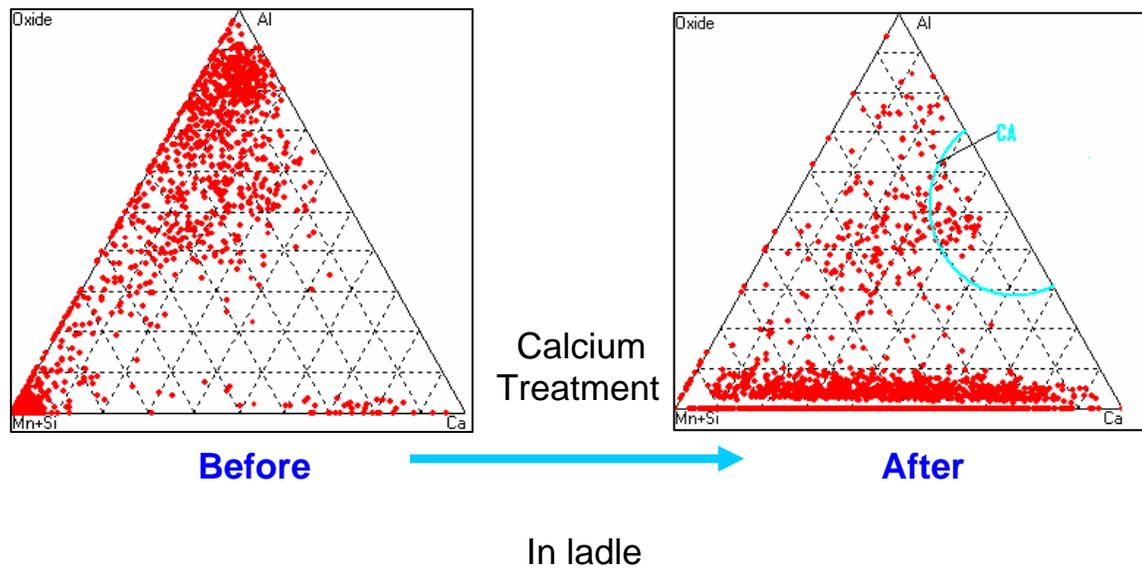
**Figure 21:** (Mn+Si)-Ca-Al composition of inclusions for basic process, before and after addition of Ca in ladle (Plant C).
