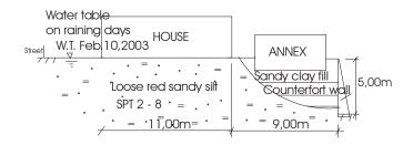
Fig. 1. Cross section of the site subsoil
