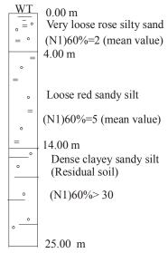
Fig. 2 Typical soil profile in the site area
