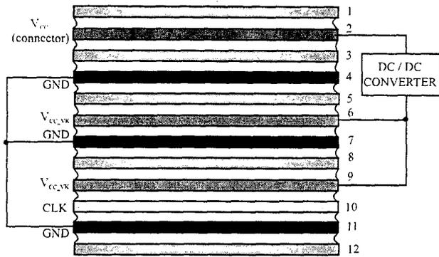
Figure 2. Layer stack-up for the CPU #1 PCB module.
