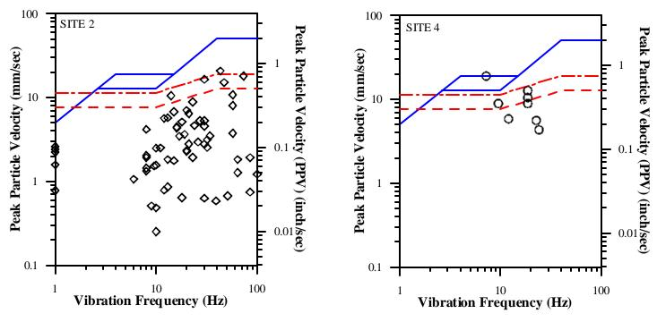
Fig. 6. PPV vs. Vibration Frequency for Site 2.
