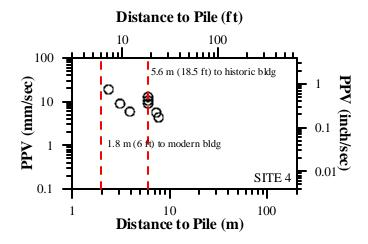
Fig. 13. PPV vs. Distance for Site 4.
