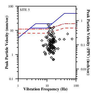
Fig. 9. PPV vs. Vibration Frequency for Site 5.
