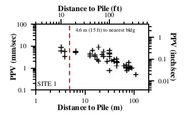
Fig. 10. PPV vs. Distance for Site 1.
