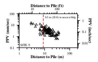
Fig. 14. PPV vs. Distance for Site 5.
