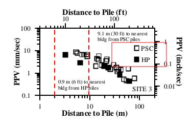
Fig. 12. PPV vs. Distance for Site 3.
