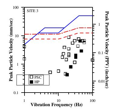
Fig. 7. PPV vs. Vibration Frequency for Site 3.
