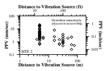
Fig. 11. PPV vs. Distance for Site 2.
