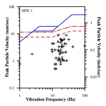
Fig. 5. PPV vs. Vibration Frequency for Site 1.
