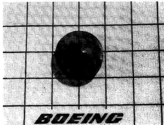
Fig. 1 Single crystal YBCO sample; grid = 1".
