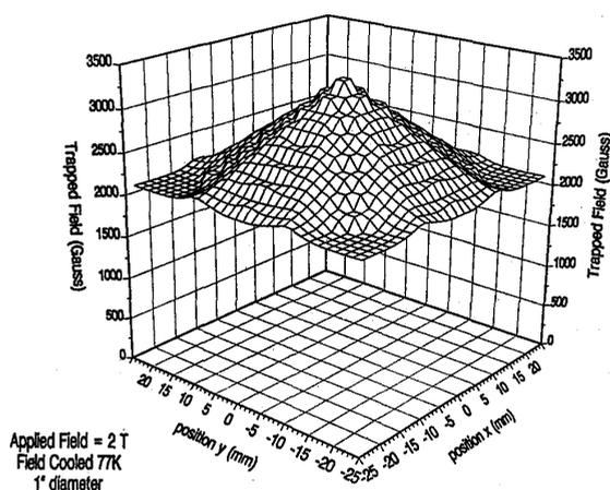
Fig. 2 Flux-trap profile of a 1"YBCO single crystal.
