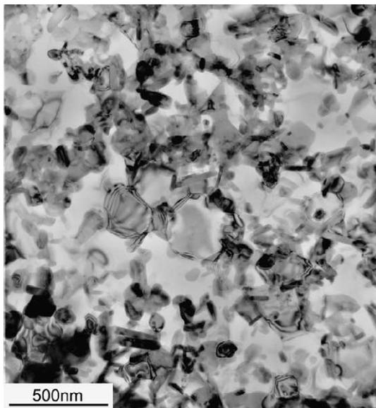
Fig. 1. Bright-field TEM micrograph of as-extruded  $\text{Al}_{89}\text{Ni}_3\text{Gd}_7\text{Fe}_1$  alloy.
