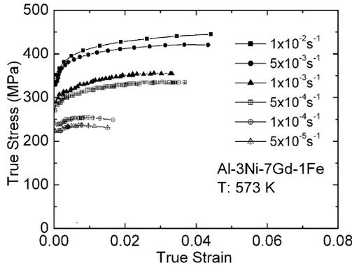
Fig. 3. Stress–strain behavior of Al<sub>89</sub>Ni<sub>3</sub>Gd<sub>7</sub>Fe<sub>1</sub> alloy at 573 K for various initial strain rates.
