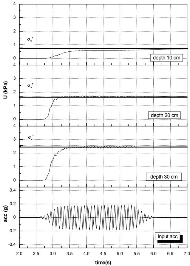
Fig. 4. Generation of pore pressure – model with no drains
