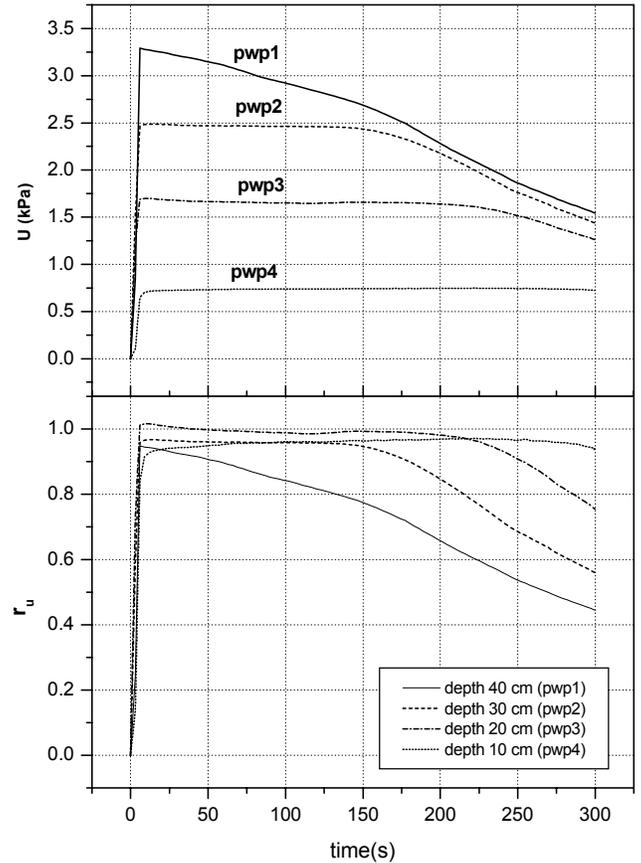
Fig. 5. Dissipation of pore pressure – model with no drains
