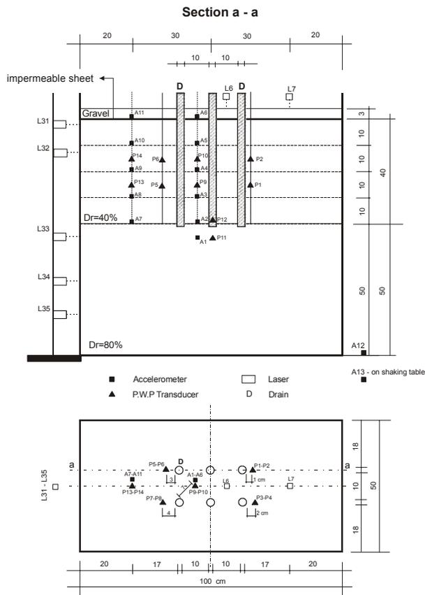
Fig. 2. Model layout and location of transducers
