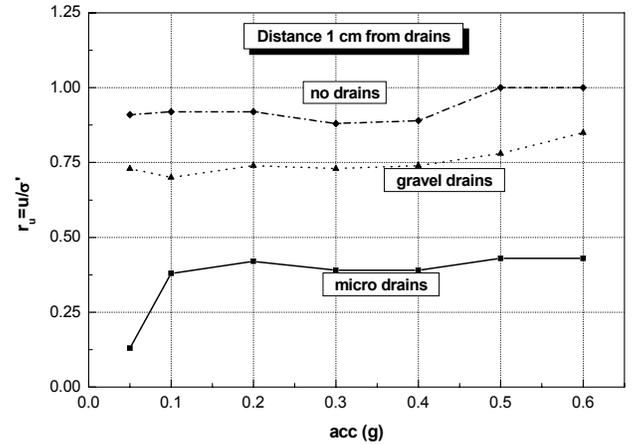
Fig. 8a. Max. excess pore pressure ratio  $r_u$  distance 1 cm from drains
