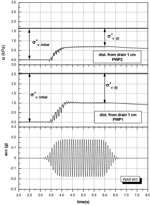
Fig. 6. Generation of pore pressure – model with micro-drains
