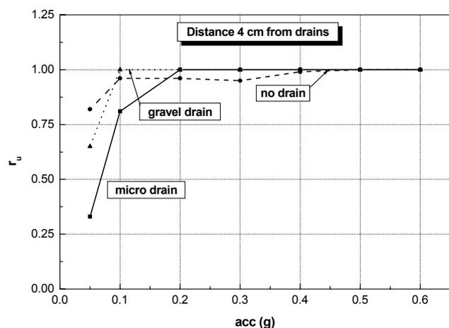
Fig. 8c. Max. excess pore pressure ratio  $r_u$  distance 4 cm from drains
