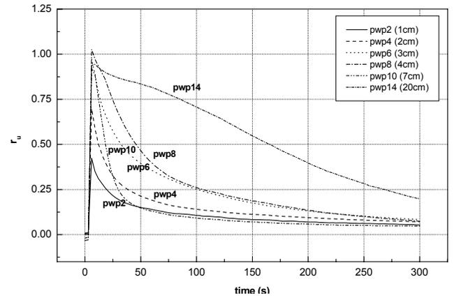
Fig. 7. Dissipation of pore pressure – model with micro-drains
