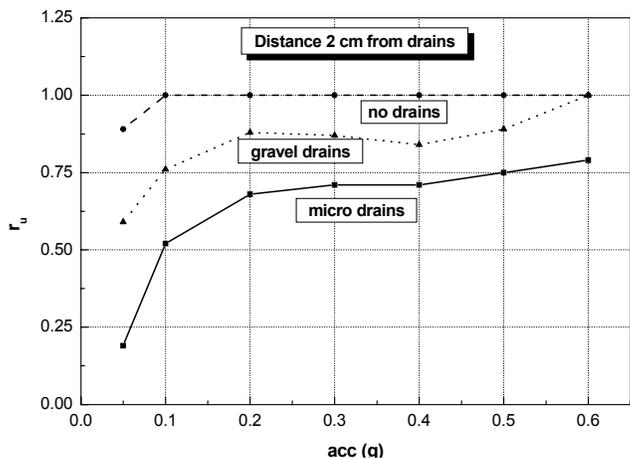
Fig. 8b. Max. excess pore pressure ratio  $r_u$  distance 2 cm from drains
