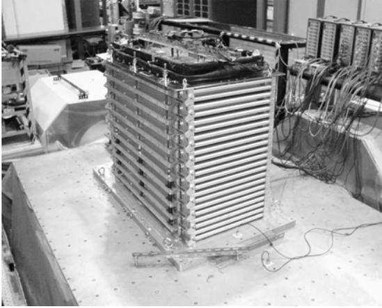
Fig. 1. Laminar box at the University of Tokyo
