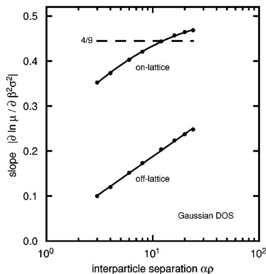
FIG. 10. The slope  $|\partial \ln \mu / \partial \beta^2 \sigma^2|$  of the data presented in Figs. 8 and 9 as a function of the mean interparticle spacing. Data labeled “off-lattice” are taken from the fits of Fig. 8, data labeled “on-lattice” are from Fig. 9. Horizontal dashed line shows the slope  $A = 4/9$  used in the disorder formalism of Ref. 4.
