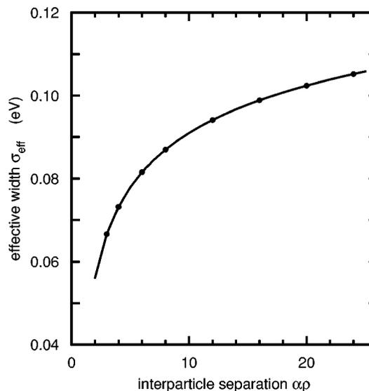
FIG. 11. Effective width  $\sigma_{\text{eff}}$  of the density of states deduced from the data of Fig. 8, assuming an actual width  $\sigma=0.14$  eV and using Eq. (6) with  $A=4/9$  to deduce  $\sigma_{\text{eff}}$ . Data are plotted as a function of the mean interparticle spacing  $\alpha\rho$ , showing an artificial concentration dependence to the density of states arising from the fitting procedure.
