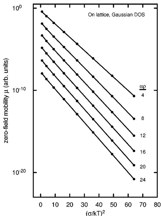
FIG. 9. Mobility  $\mu$  as a function of the dimensionless parameter  $\hat{\sigma}^2 = (\sigma/kT)^2$  for a system with a Gaussian density of states of width  $\sigma$ , parametric in the mean interparticle spacing  $\alpha\rho$ . Transport sites are located on an ordered and filled lattice with unit cell spacing  $\rho$ . Computed data are represented by filled circles, straight lines are numerical fits.
