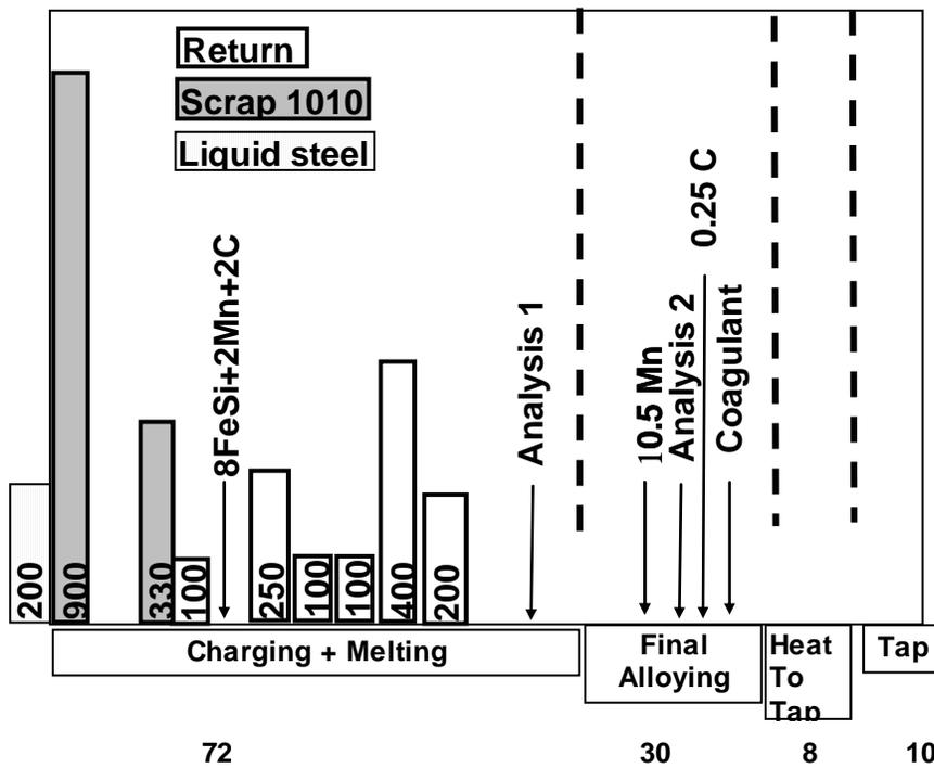
Figure 1. Time-operational graph of melting steel in hot induction furnace with 200 lb heel (Foundry A)
