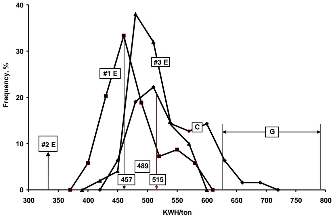
Figure 17. Variation of electrical energy consumption for steel melting in EAF
