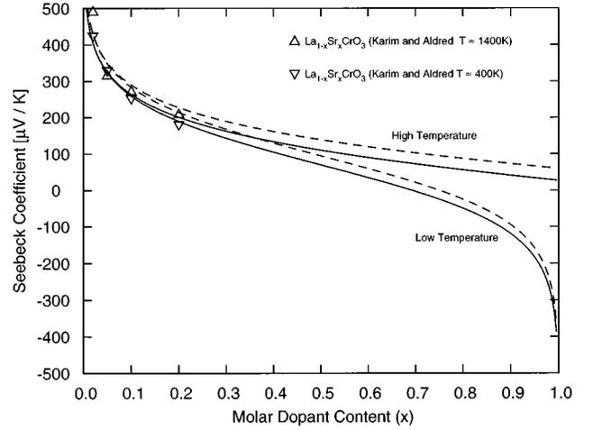
FIG. 3. Predicted high- and low-temperature limits of the Seebeck coefficient as a function of acceptor doping calculated for the  $\text{La}_{1-x}\text{Sr}_x\text{CrO}_3$  series. Experimental data are from the study of Karim and Aldred (Ref. 8) for  $\text{La}_{1-x}\text{Sr}_x\text{CrO}_3$  at high and low temperatures as indicated. Solid lines indicate predictions for weak magnetic coupling, dashed lines for strong magnetic coupling.
