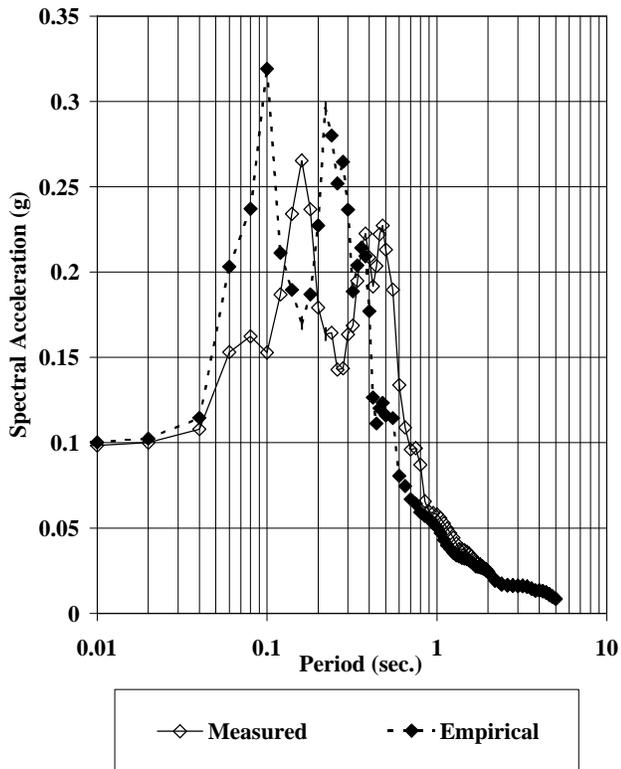
Figure 7 - Response Spectra at 5 ft. BGS - Site 5
