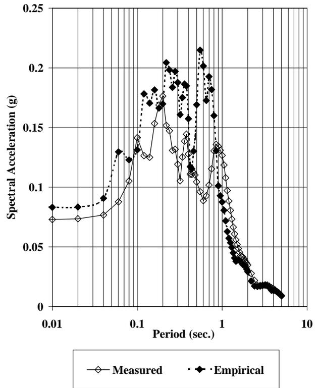
Figure 9 - Response Spectra at 5 ft. BGS - Site 8
