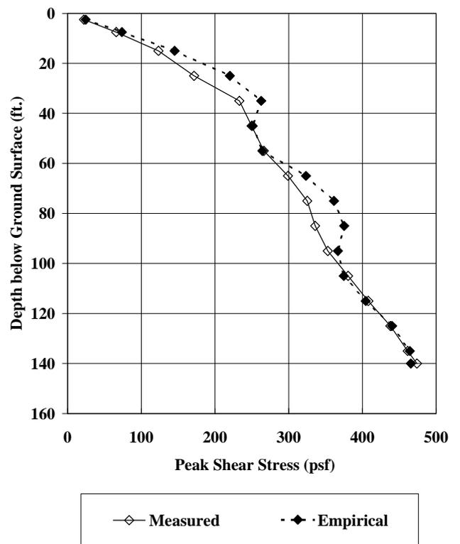
Figure 13 - Shear Stress Curve - Site 8
