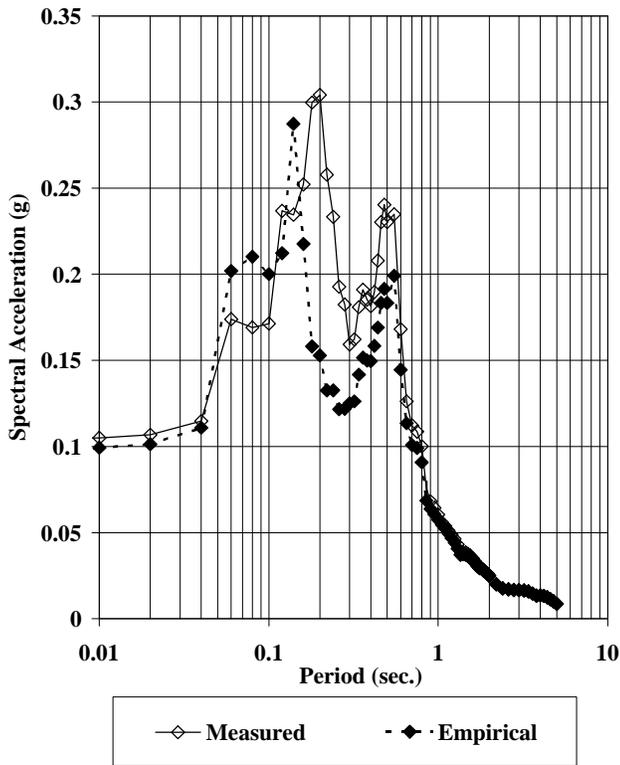
Figure 6 - Response Spectra at 5 ft. BGS - Site 3
