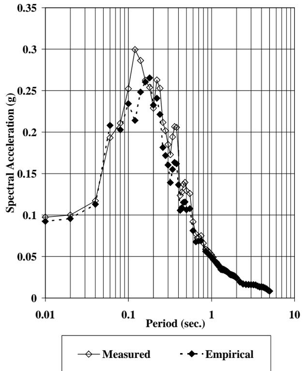
Figure 8 - Response Spectra at 5 ft. BGS - Site 7
