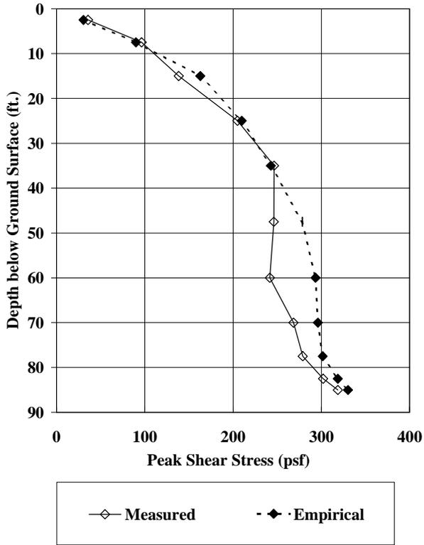
Figure 10 - Shear Stress Curve - Site 3
