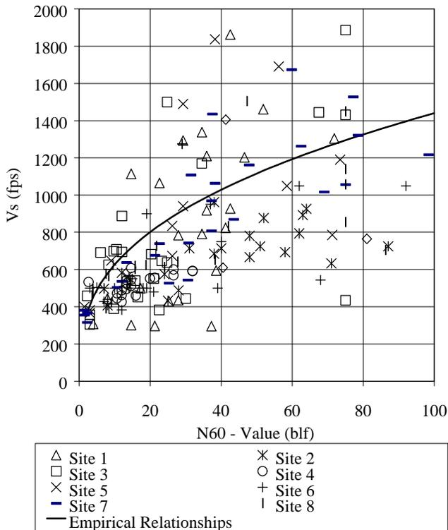
**Figure 1 - Comparison of Measured and Empirically Derived Shear Wave Velocities**
