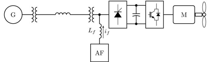
Fig. 4. Active filter connection to a shipboard power system.
