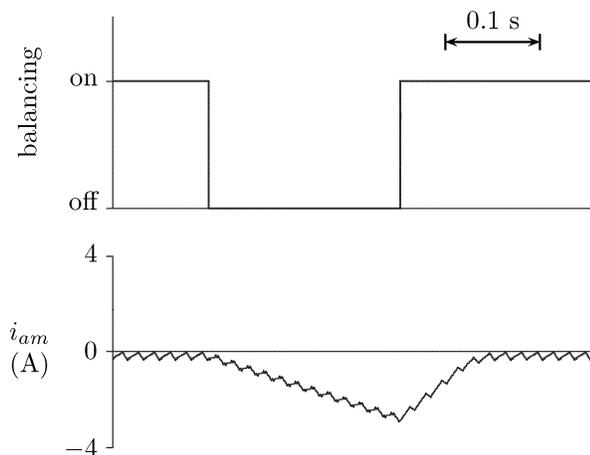
Fig. 8. Magnetizing current with and without balancing algorithm.
