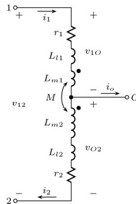
Fig. 3. Detailed model of the tapped reactor.
