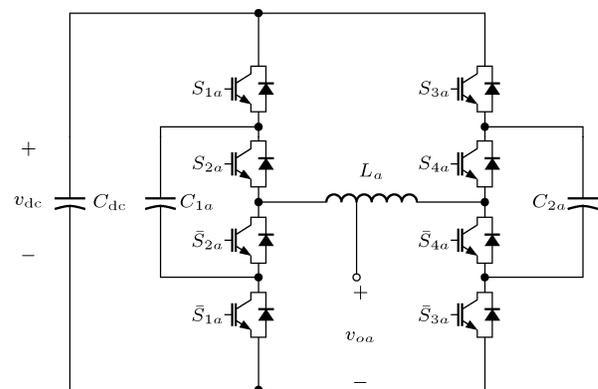
Fig. 1. Phase  $a$  of the seven-level active filter topology.
