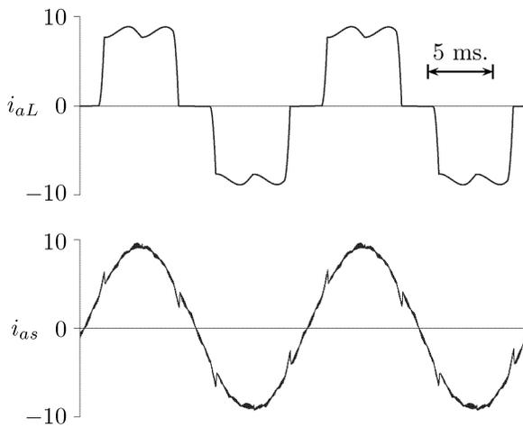
Fig. 7. Load current and compensated current.
