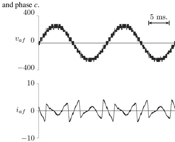
Fig. 6. Active filter output voltage and current.
