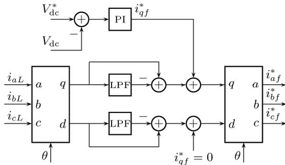
Fig. 5. Active filter control diagram.
