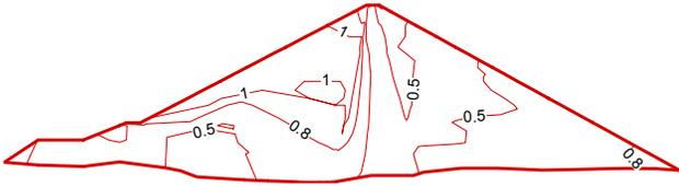
Fig. 10. Mobilized shear stress level contours
