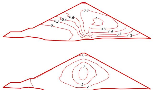
Fig. 7. Deformation contours (m). (a) Horizontal direction, (b) Vertical direction
