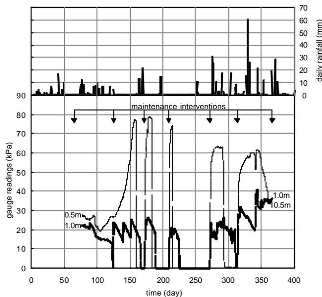
Figure 2. Rainfall characteristics and suction response at site B during year 2000: rainfall gauge readings and matric suction measurements at 0.5 e 1.0m depths.
