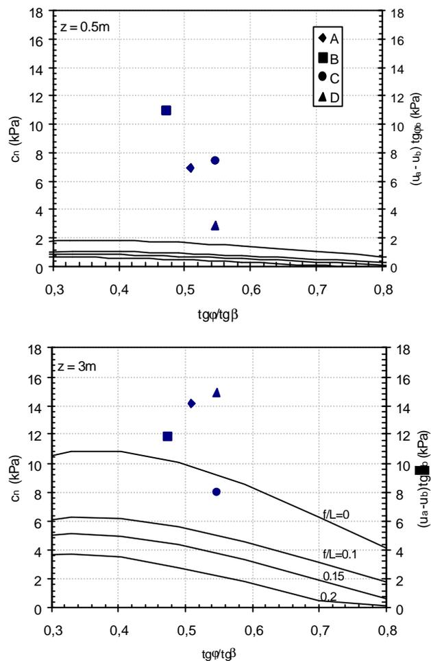
Figure 5. Cohesion necessary  $c_n$  e apparent cohesion during the rainy season: for  $z=0,5$  and for  $z=3\text{m}$ .
