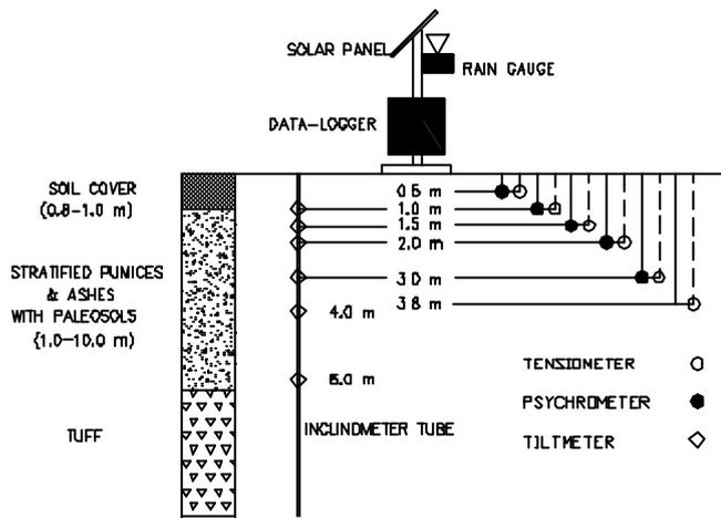
Figure 1. Sketch of a typical soil profile and instrumentation layout.
