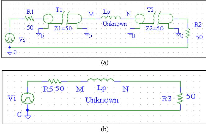
Figure 7. Equivalent circuit for edge-launch transition measurement.
