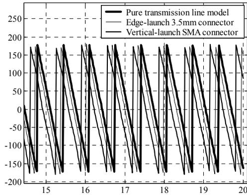
Figure 11.  $S_{21}$  phase comparison for different launch techniques.
