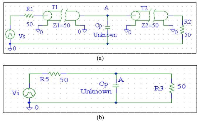
Figure 8. Equivalent circuit for vertical-launch transition measurement.
