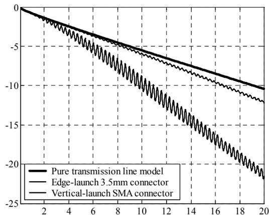
Figure 10.  $|S_{21}|$  comparison for different launch techniques.
