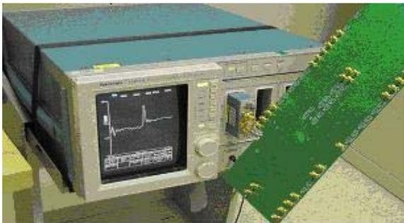
Figure 2. Measurement setup for edge-launch port without compensation.
