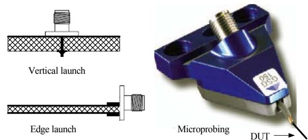
Figure 1. Three main wave-launch methods.
