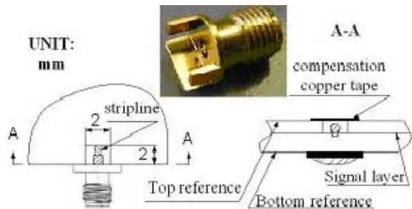
Figure 6. Schematic edge-launch structure and port compensation.
