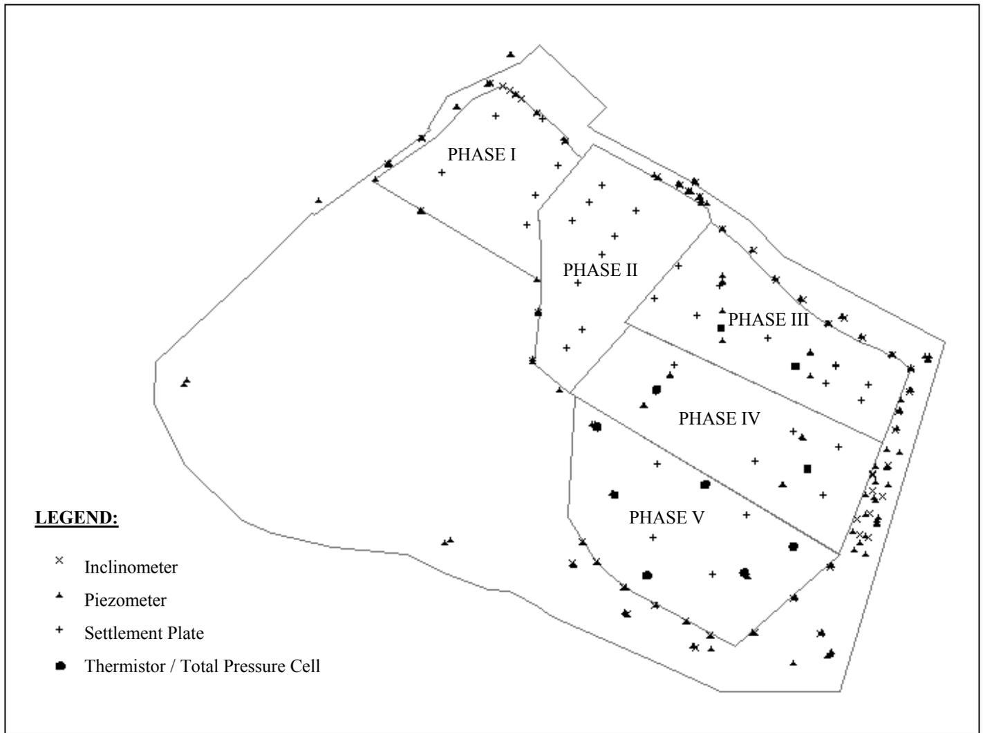
Fig. 3. Instrumentation Location.
