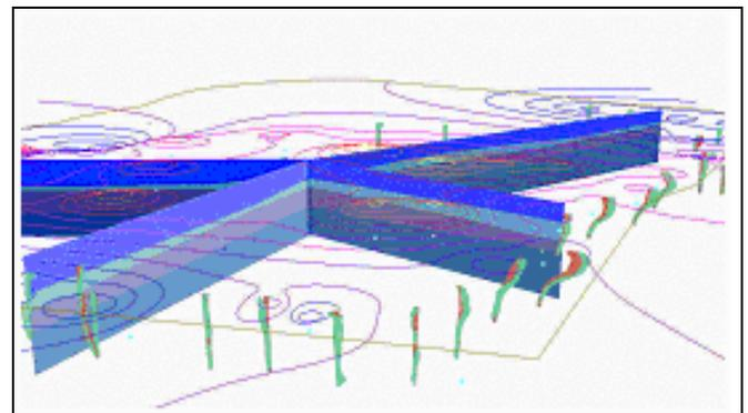
Fig. 5. Typical Fence Diagram.
