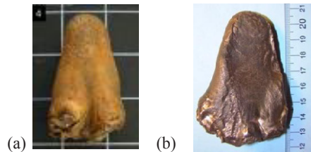
Fig. 8. Illustrates the damage imparted on the projectile from impacting the third polyethylene segment by comparing a projectile from Method 2 (a) with a flattened projectile from Method 1 (b).
