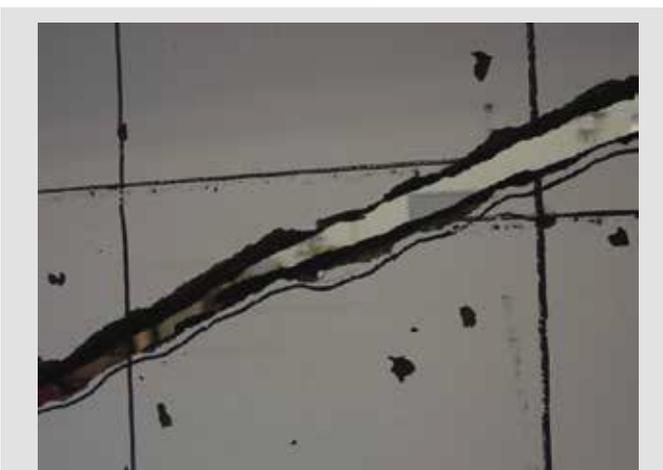
**Figure 6.** Shear crack in girder 2 from test 2.
