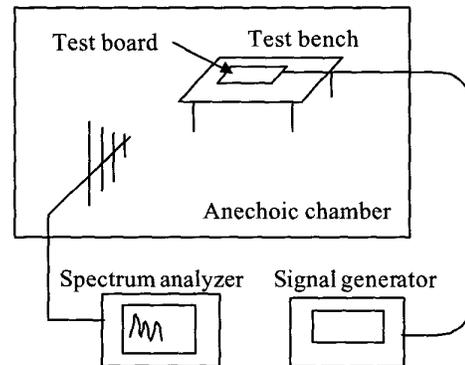
Fig. 5. Setup for measuring the radiated fields.
