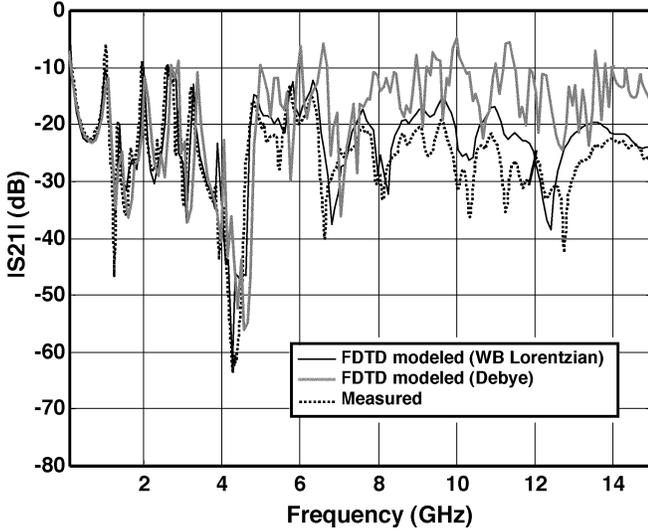
Fig. 6. Measured and FDTD modeled  $|S_{21}|$  frequency dependence for a composite material as the WBL dielectric with the parameters  $\epsilon_s = 2.5$ ,  $\epsilon_\infty = 2.15$ ,  $\Delta f = 190$  GHz,  $f_0 = 85$  GHz, and as the Debye dielectric with the parameters  $\epsilon_s = 2.5$ ,  $\epsilon_\infty = 2.15$ ,  $\tau_r = 2.5 \cdot 10^{-12}$  s. Conductivity in both cases was taken as  $\sigma_e = 10^{-4}$  S/m.
