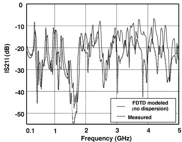
Fig. 3. Measured and FDTD modeled scattering matrix parameter  $|S_{21}|$  for the test substrate without taking into account a dispersive nature of a dielectric,  $\epsilon_r = \text{const} = 4.3$  and  $\sigma_e = 4 \cdot 10^{-3}$  S/m.
