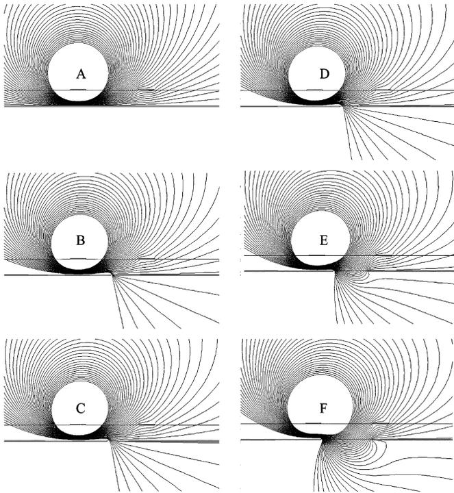
Fig. 11. Contour maps of the magnetic flux from test boards with varying width gaps in the return plane. (a) No gap. (b)  $w_{\text{gap}} = 0.025$  cm. (c)  $w_{\text{gap}} = 0.076$  cm. (d)  $w_{\text{gap}} = 0.127$  cm. (e)  $w_{\text{gap}} = 0.305$  cm. (f)  $w_{\text{gap}} = 0.381$  cm.
