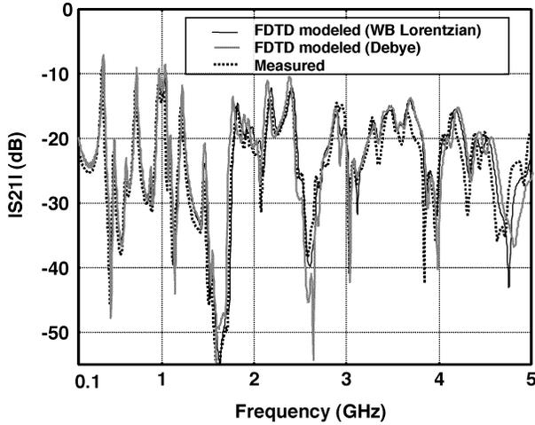
Fig. 5. Measured and FDTD modeled  $|S_{21}|$  for the test substrate as a WBL dielectric with the parameters  $\epsilon_S = 4.301$ ,  $\epsilon_\infty = 4.096$ ,  $\sigma_e = 2.294 \cdot 10^{-3}$  S/m,  $f_0 = 39.5$  GHz, and  $\Delta f = 200$  GHz, and as a Debye dielectric with the parameters  $\epsilon_S = 4.301$ ,  $\epsilon_\infty = 4.096$ ,  $\sigma_e = 2.294 \cdot 10^{-3}$  S/m, and  $\tau_r = 2.321 \cdot 10^{-11}$  s.
