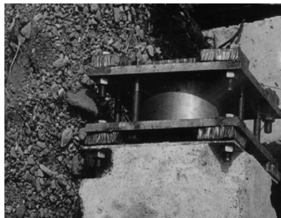
Fig. 3. A strain-gauge dynamometer with a circular measuring element
