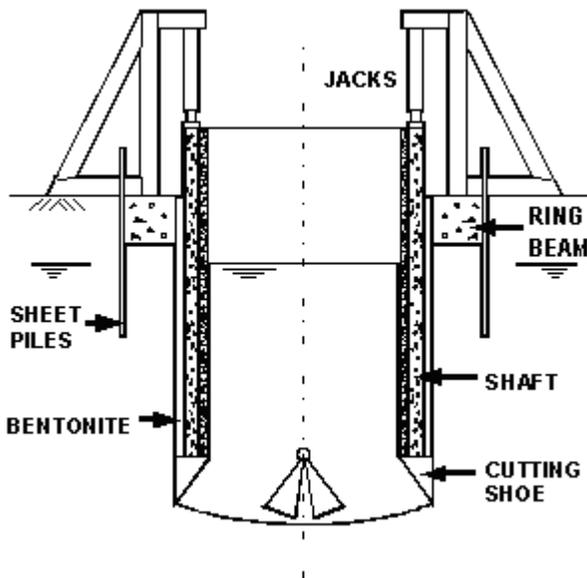
Fig. 8. Seal chamber bolted segmental caisson installation for sea outfall, Site C (after Heavey, et al., 2000)
