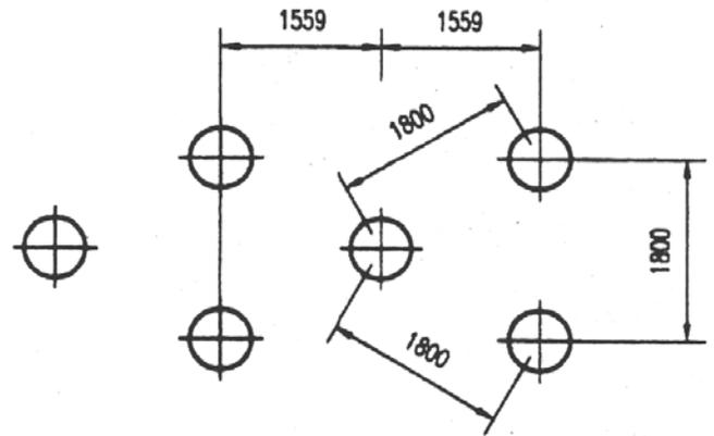
Fig. 11. Stone column layout pattern, for 150kN/m<sup>2</sup> bearing capacity, Site D in Lincolnshire
