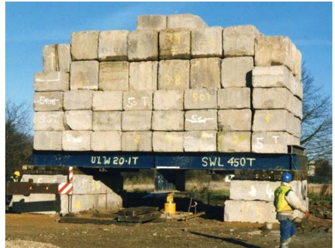
Fig. 12. Zone test on 150kN/m<sup>2</sup> Stone column layout
