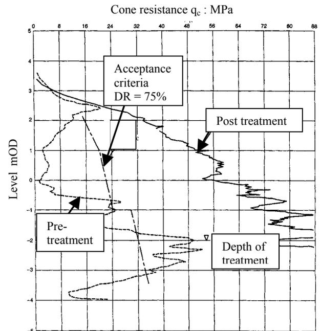
Fig. 9. Pre and post treatment CPT performance data and acceptance criteria, Site C. (after Slocombe et al., 2000)
