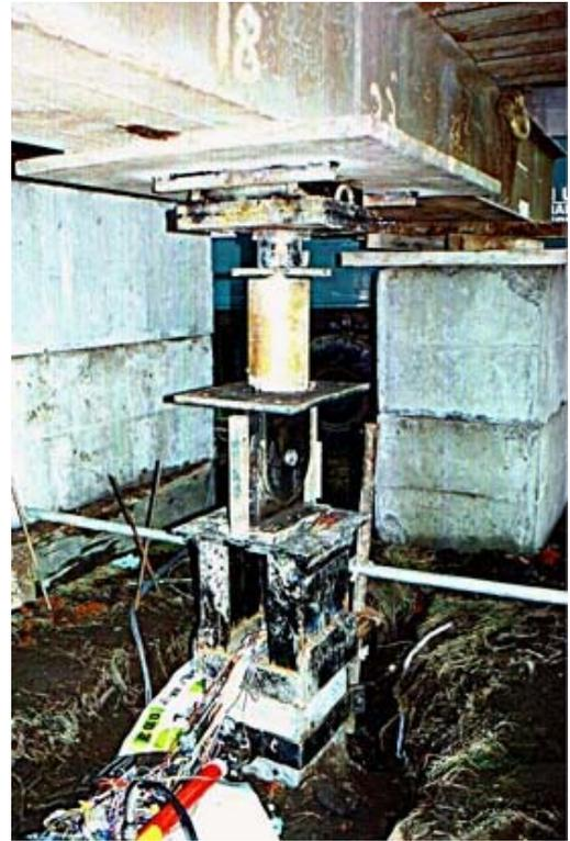
Fig. 4: Test setup at pile AL1
