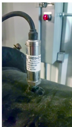
Fig. 6. Omegadyne PX409 pressure sensor installed on 38 L chamber.
