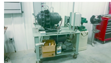
Fig. 4. Explosive chamber used in flame extinguishing experiment.
