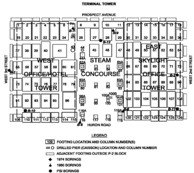
Fig. 3. General arrangement of footings in P-2 Block
