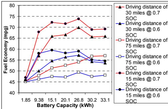
Figure 6. Battery capacity vs. fuel economy for initial SOC greater than 0.5
