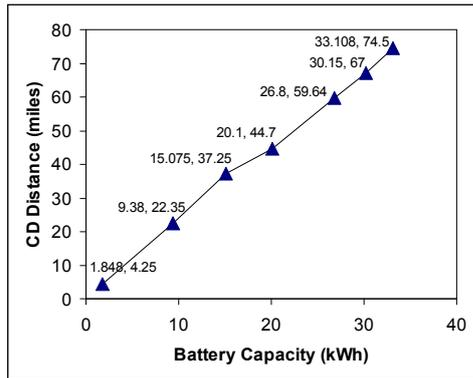
Figure 2. Battery capacity vs. CD Distance @ 0.7 SOC
