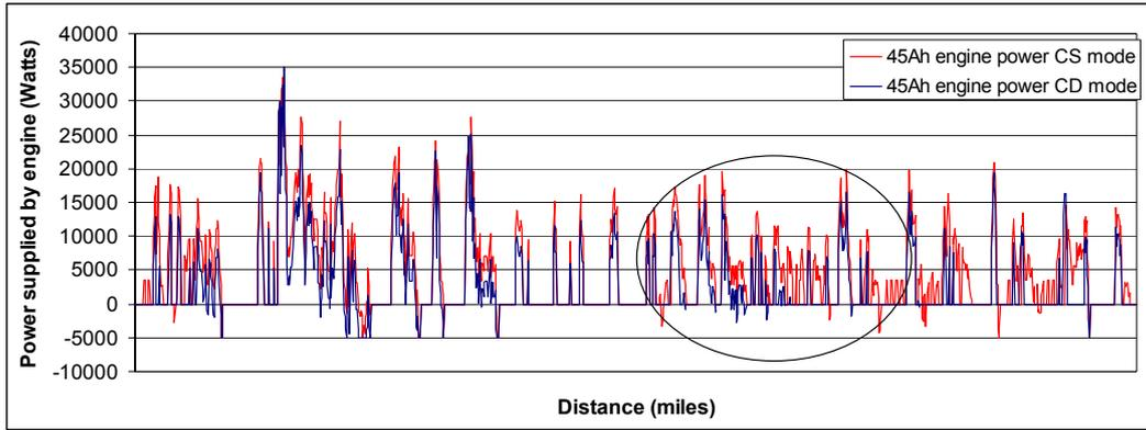
Figure 4. Power supplied by the engine during the beginning (CD mode) and at the end of drive cycle (CS mode)
