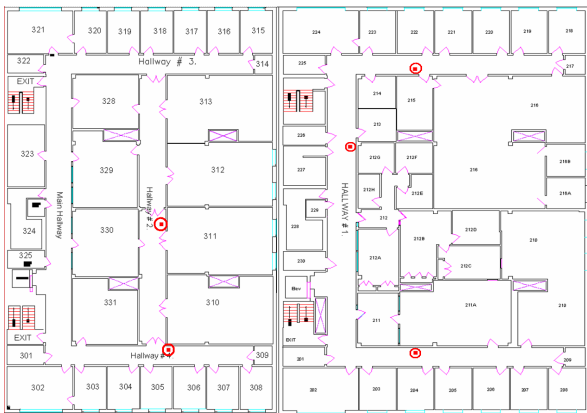
Fig. 5. Floor plans of ERL third and second floor. Receiver pair positions are marked with circled squares. Transmitter positions are evenly distributed on the hallways on both floors.
