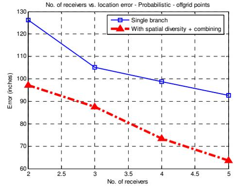
Fig. 6. Probabilistic Technique : Location error as a function of number of receivers.
