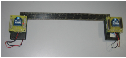
Fig. 4. UMR-SLU G4-SSN motes arranged for creating spatial diversity with a separation of 25 cms
