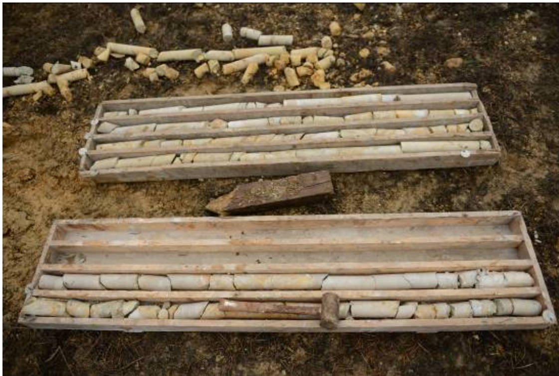
Figure 5: The rock core from Site 1.
