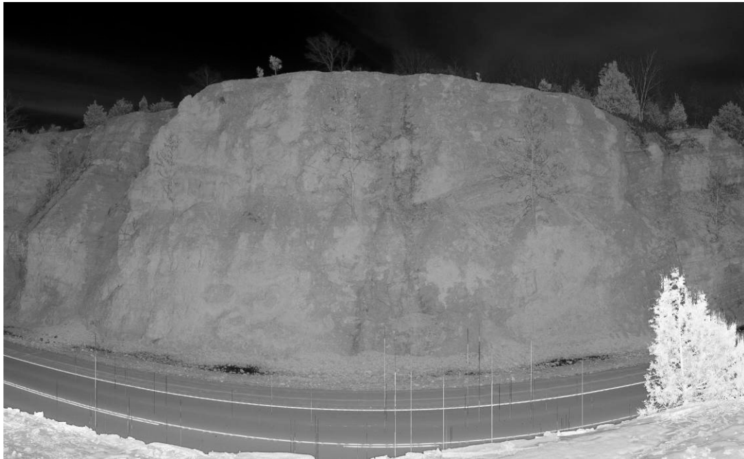
Figure 13: Scanning result. Vertical lines show when the scanner intercepted cars speeding done the highway. These are easily edited out.
