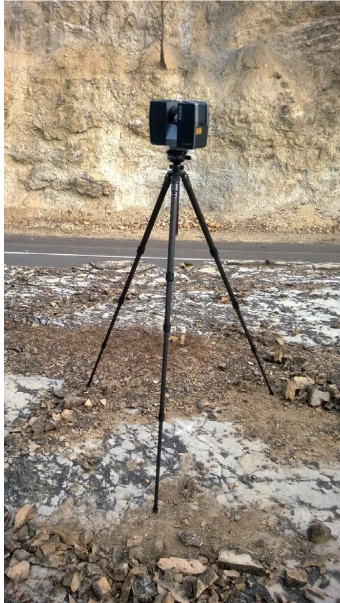
Figure 12: LIDAR scanning, site 1.
