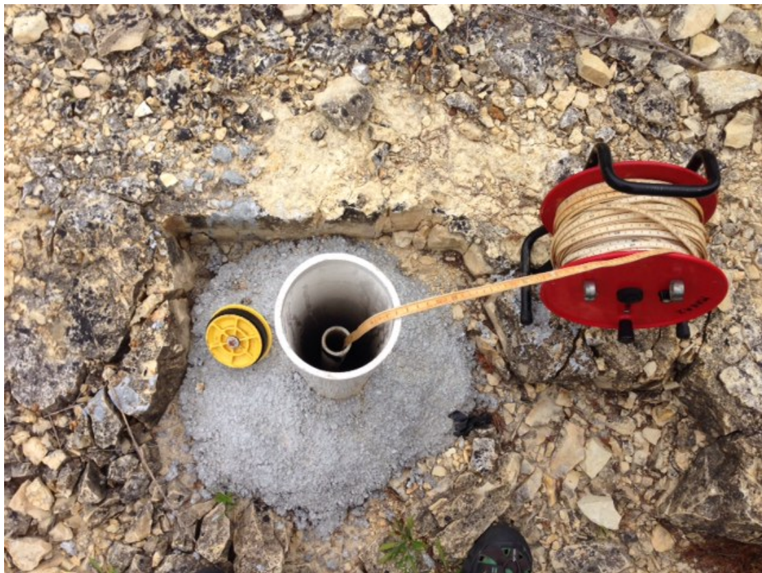
Figure 7: Making water level measurements.
