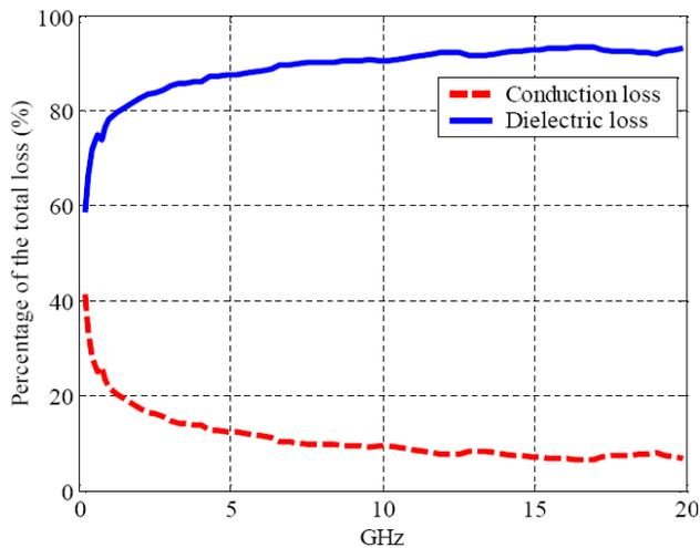
Figure 5. Quantified dielectric loss and conductor loss.
