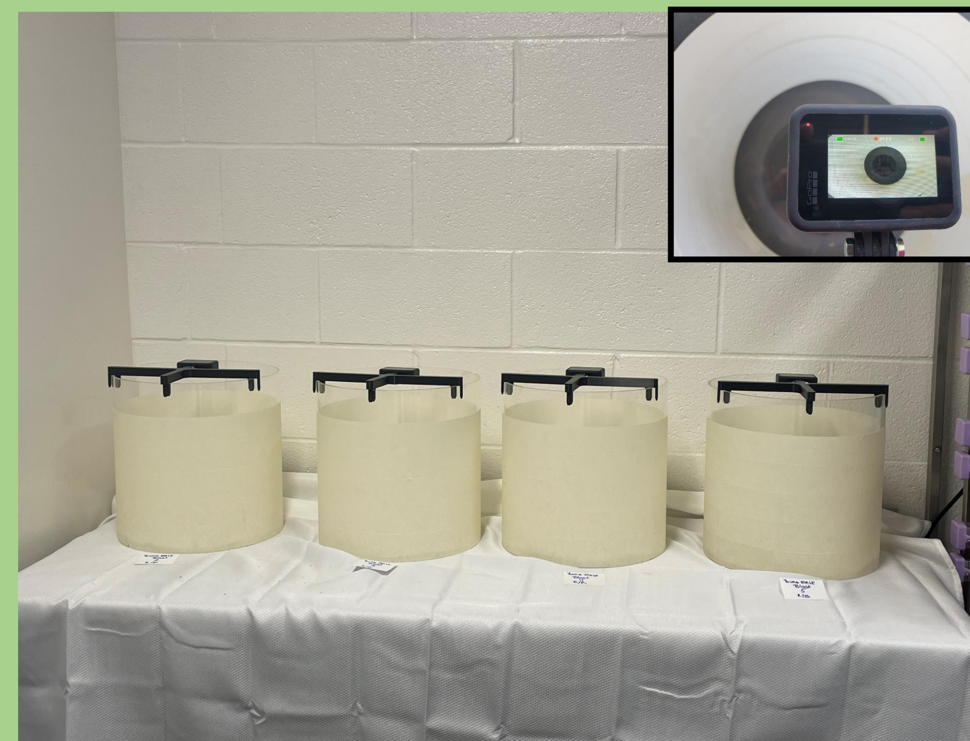
Fig 5. Custom built chambers using GoPro mounts on top for video recording mice. Insert: GoPro camera set-up looking into chambers.
