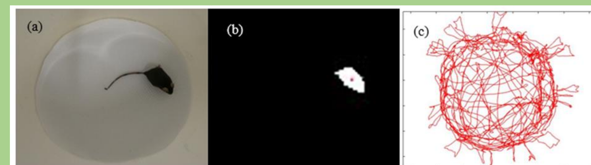
Fig 7. Protocol to video record and analyze mouse movement with MATLAB. (a) still frame of a mouse in the recoding cage. (b) computer adaptation (c) data points for the mouse movement during 5-minute video
