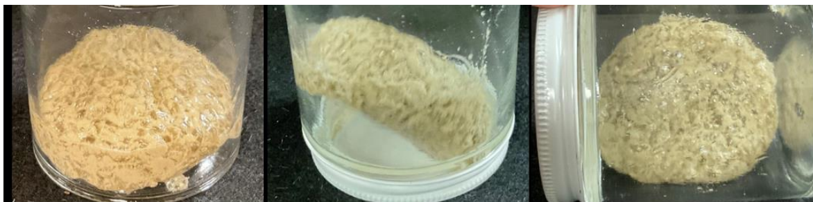
Figure 2 Clumping Effect recorded at 1/10 RPPG ratio, 7% Bentonite, 2% KCl, and 0.2% Fiber concentration
