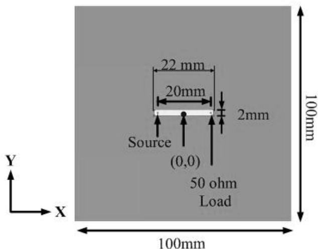
Figure 4. Front view of the measured microstrip structure.
