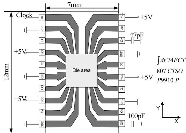
Figure 10. The clock buffer and its connections.
