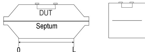
Figure 1. Cross sections of a TEM cell.
