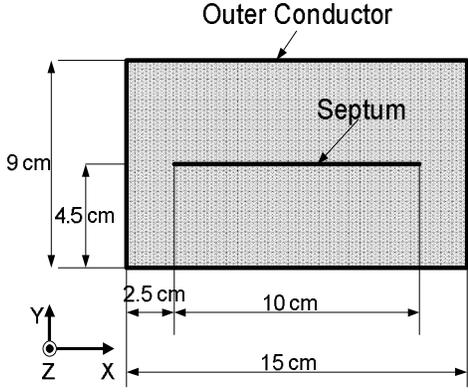
Figure 2. Detailed cross-section of the TEM cell.
