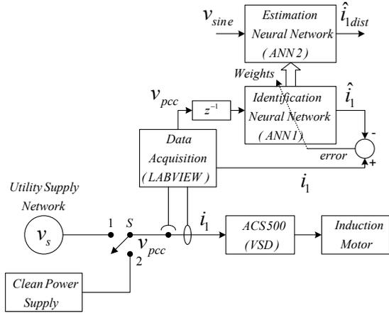
Fig. 4: Experimental Setup for ACS 500 Drive
