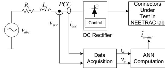
Fig. 13: Experimental Setup for RXPO Series 30 Rectifier
