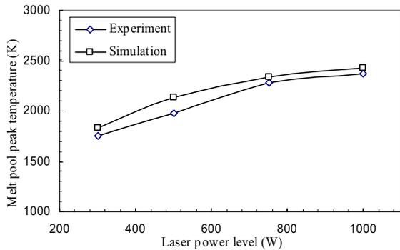
**Fig. 8. Melt pool peak temperature comparison between simulation and experiment at different laser power level.**
