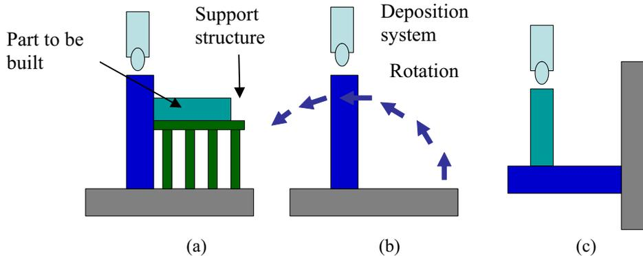
**Fig 1. (a) build part with support structure; (b) with multi-axis capability, after building the column, the table can be rotated; (c) After rotation, continue to build the component from another direction.**
