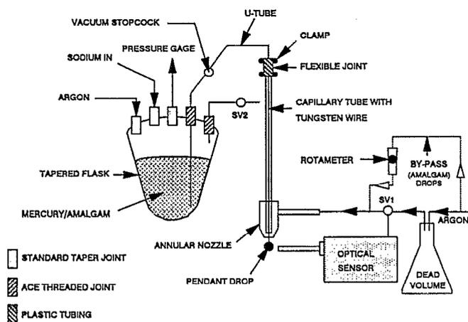
FIG. 2. Schematic diagram of the single drop apparatus.
