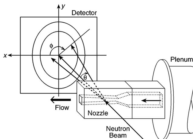
FIG. 2. The aerosol is formed in the nozzle which sits in the neutron beam. The scattering angles  $\theta$  and  $\phi$  are defined. Two contour lines of constant scattering intensity are shown on the detector.
