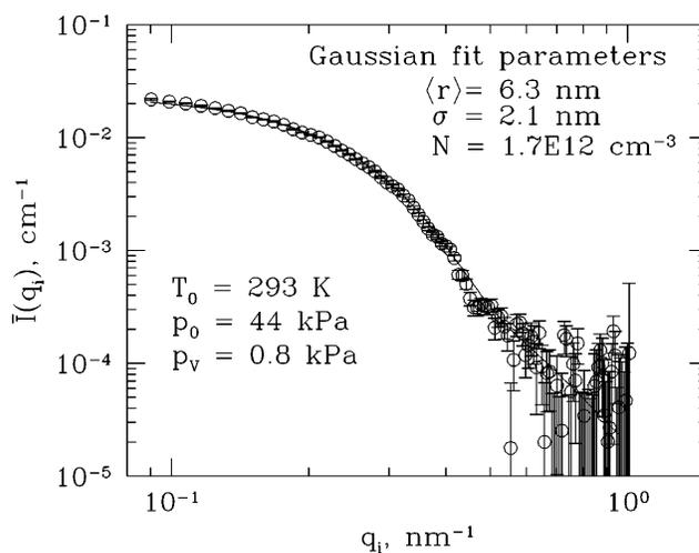
FIG. 4. The SANS spectrum for D<sub>2</sub>O nanodroplets in the supersonic nozzle for experiment 1. The solid line is calculated for a droplet distribution with the parameters shown.
