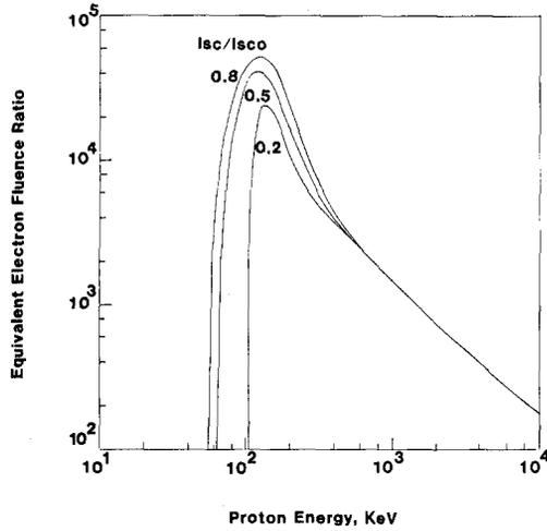
Fig. 3. Equivalent electron fluence ratio for GaAs heteroface solar cells with an  $0.4\text{-}\mu\text{m}$  (GaAl)As window and  $0.5\text{-}\mu\text{m}$  junction depth as a function of proton energy for three different damage levels.
