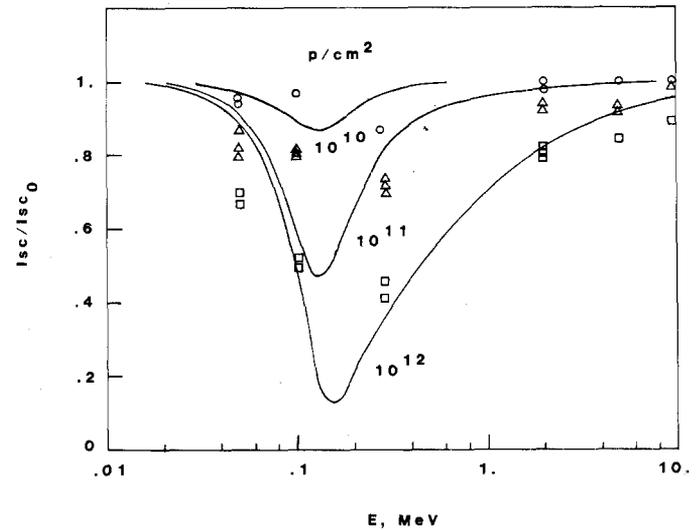
Fig. 2. Reduced short-circuit current for monoenergetic proton exposure at three fluence levels. Experimental data are noted as  $\circ$  for  $10^{10} \text{ p/cm}^2$ ,  $\Delta$  for  $10^{11} \text{ p/cm}^2$ , and  $\square$  for  $10^{12} \text{ p/cm}^2$ .
