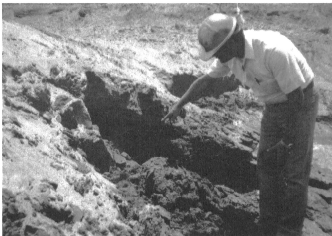
Fig.9 Detail of thin layers of peat and organic clay
