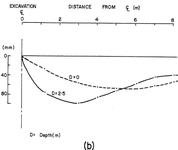
Figure 3. Soil displacements due to effect of excavation at different depths and distances from centre line. (a) vertical movements. (b) lateral movements.
