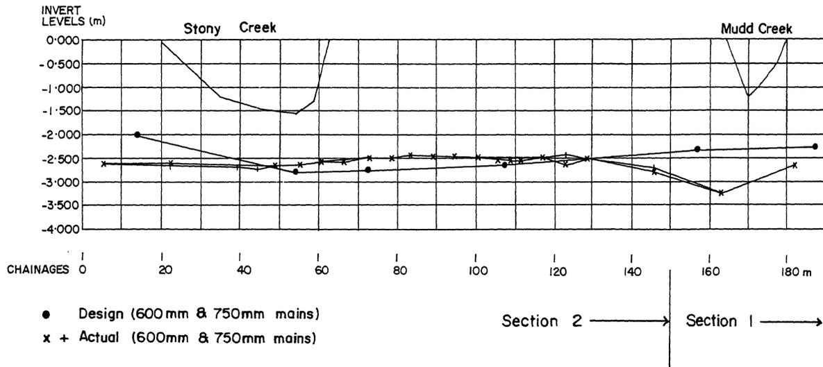
Figure 4. Design and actual position of mains.
