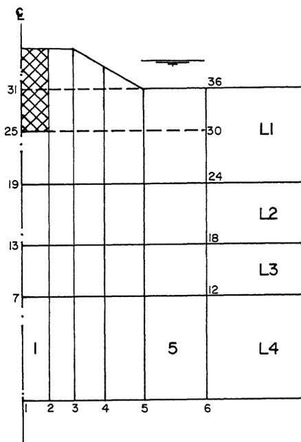
Figure 1. Finite layer and nodes used for analysis (sublayers are not shown).
