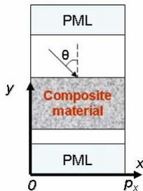
Figure 2. The side view of a unit element of periodic structure for FDTD simulation.
