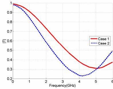
Figure 13. Transmission coefficient versus frequency for various inclusions (normal incidence).
