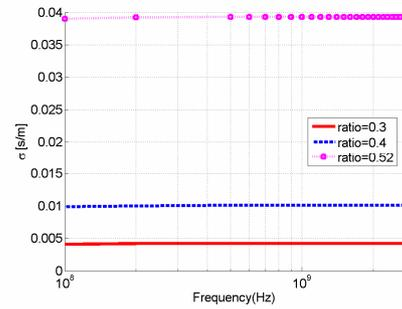
Figure 5. Effective conductivity versus frequency for various radius of spherical inclusion.
