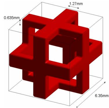
Figure 9. A unit cell for the third example.
