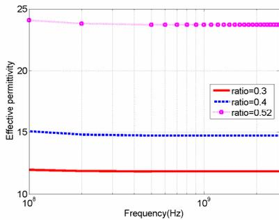
Figure 4. Effective relative permittivity versus frequency for various radius of spherical inclusion.
