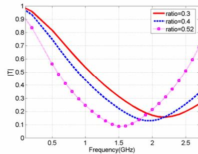
Figure 7. Transmission coefficient versus frequency for various radius of spherical inclusion (normal incidence).
