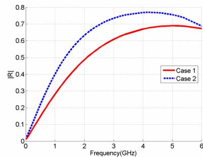
Figure 12. Reflection coefficient versus frequency for various inclusions (normal incidence).
