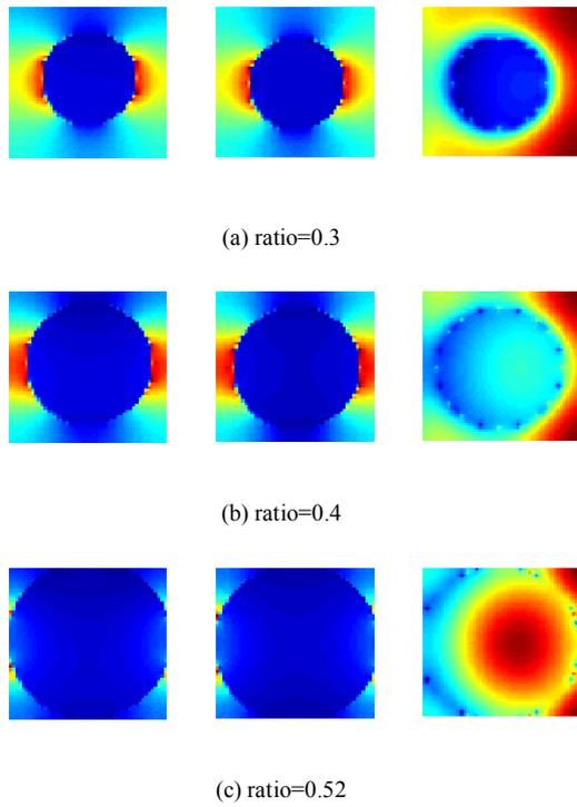
Figure 8. Normalized electric fields along three center-cut planes.
