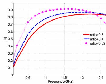
Figure 6. Reflection coefficient versus frequency for various radius of spherical inclusion (normal incidence).
