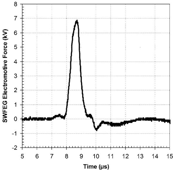
FIG. 3. Wave form of the pulsed electromotive force produced by a SWFEG operating in the open circuit mode. PZT energy-carrying element had dimensions of  $D=27$  mm/ $h=2.1$  mm.
