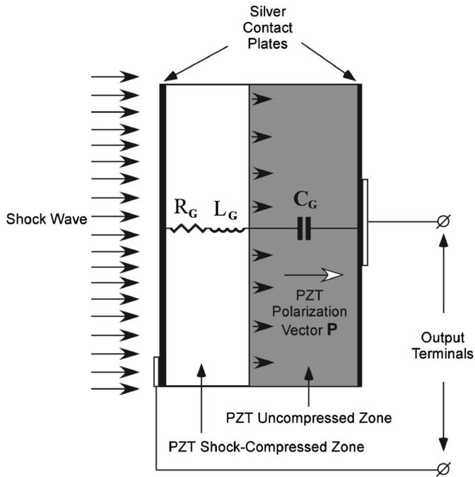
FIG. 1. Schematic diagram illustrating operation of the shock-wave ferroelectric generator.  $R_G$  and  $L_G$  are the resistance and inductance, respectively, of the shock-compressed zone of the ferroelectric energy-carrying element (through which the shock wave has already passed).  $C_G$  is the capacitance of the uncompressed zone (through which the shock wave has not passed).
