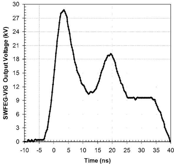
FIG. 5. Wave form of a typical high-voltage pulse produced by an explosive-driven SWFEG-VIG system. The SWFEG contained a PZT disk of dimensions  $D=27$  mm/ $h=2.1$  mm. The VIG contained eight turns, and its spark gap breakdown voltage was 2.6 kV.
