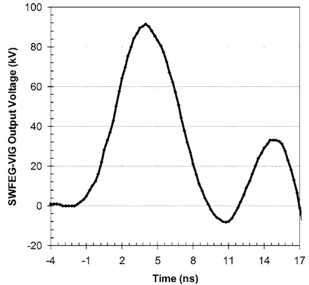
FIG. 7. Wave form of a typical high-voltage pulse produced by an explosive-driven SWFEG-VIG system. The SWFEG contained a PZT disk of dimensions  $D=25$  mm/ $h=5.1$  mm. The VIG contained five turns. The VIG spark gap breakdown voltage was 11.1 kV.
