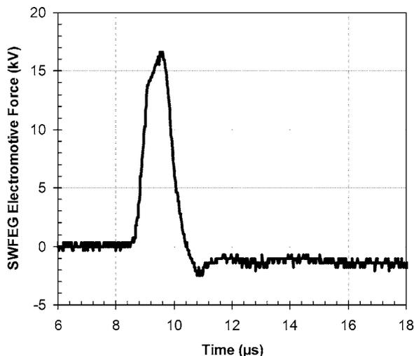
FIG. 6. Wave form of the pulsed electromotive force produced by a SWFEG operating in the open circuit mode. PZT energy-carrying element had dimensions of  $D=25$  mm/ $h=5.1$  mm.
