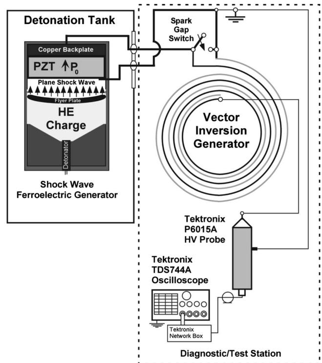
FIG. 2. Schematic diagram of a completely explosive SWFEG-VIG system.
