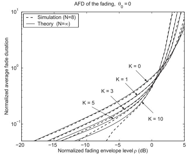
Fig. 9. The normalized AFD of the fading envelope  $|Z(t)|$ , where  $\theta_0 = 0$  for all  $K > 0$  Rician fading.
