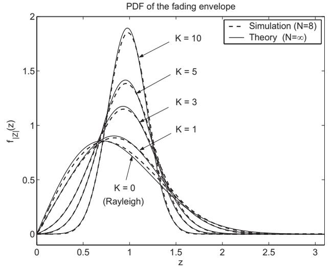
Fig. 6. The PDF of the fading envelope  $|Z(t)|$ .
