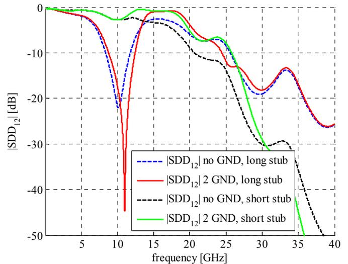
Figure 6. Differential insertion loss for short and long stub cases with and without GND vias.
