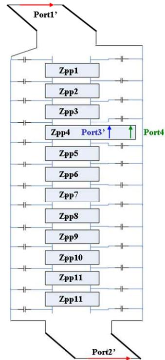
Figure 8. Simplified equivalent circuit with differential ports.
