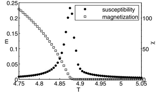
FIG. 1. Magnetization and susceptibility ( $L = 100$ ,  $c = 0.2$ ).
