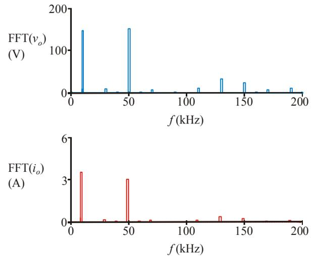
Figure 18. Unequal source 4-step, 5-level inverter output spectrums.
