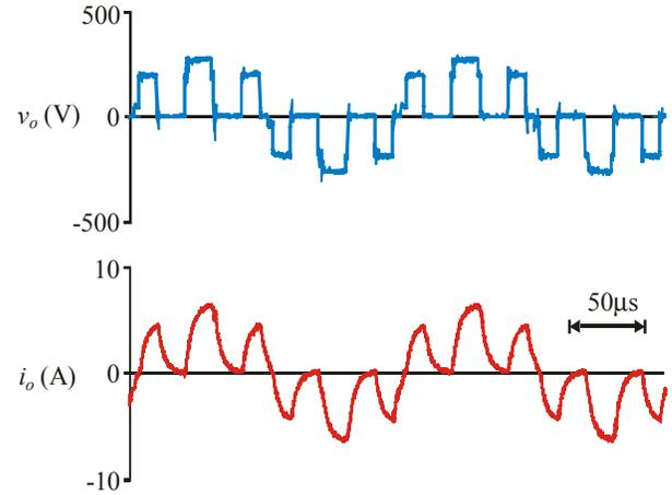
Figure 17. Unequal source 4-step, 5-level inverter waveforms.
