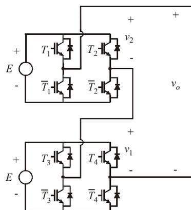
Figure 1. Cascaded H-bridge (2-cell) multilevel converter circuit
