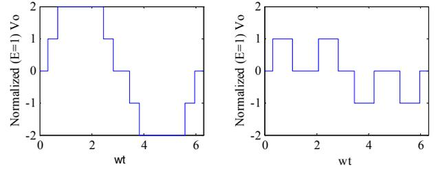
Figure 3. 2-step waveform alternatives (PP and PN)
