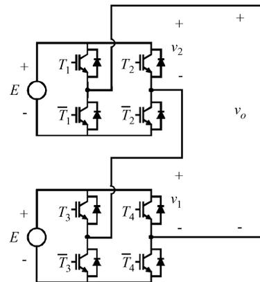
Fig. 1. Cascaded H-bridge (two-cell) multilevel inverter circuit.
