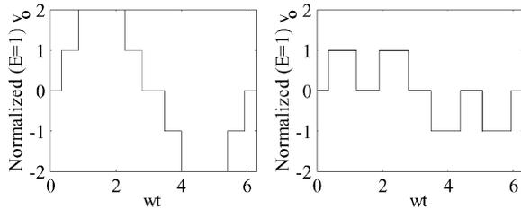
Fig. 2. Two-step waveform alternatives (PP and PN).
