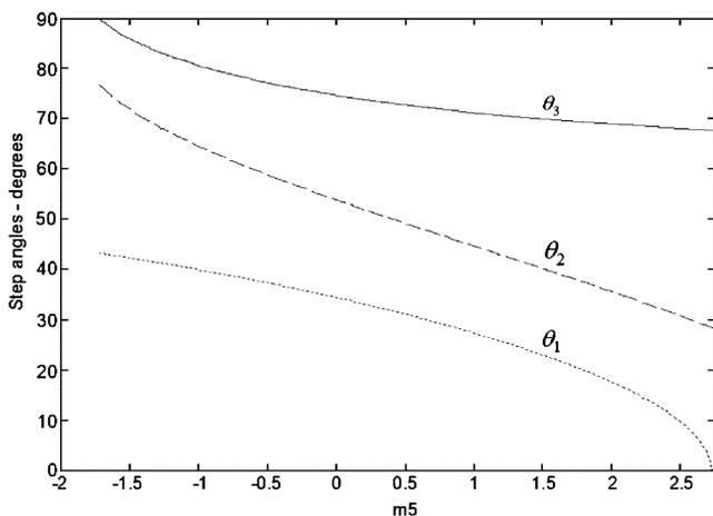
Fig. 8. Step angle solutions for  $m_1 = 0.5$  (PNP case).
