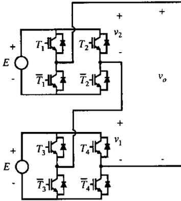
Fig. 1. Cascaded H-bridge (2-cell) multilevel converter circuit
