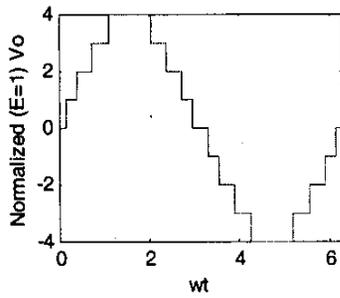
Fig. 2. 4-step, 9-level waveform
