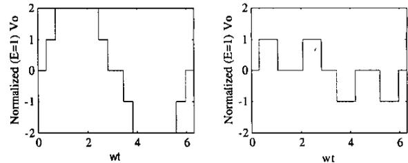
Fig. 3. 2-step waveform alternatives (PP and PN)
