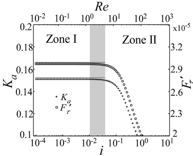
**Figure 2.** The deviation from Darcy's law shown by the non-linearity in apparent hydraulic conductivity  $K_a$  [m/s] and rate of change in friction drag [N] at increasing hydraulic gradient  $i$  [–]. Zone I shows where Darcy's law is valid and Zone II marks the emergence of the Forchheimer flow regime.
