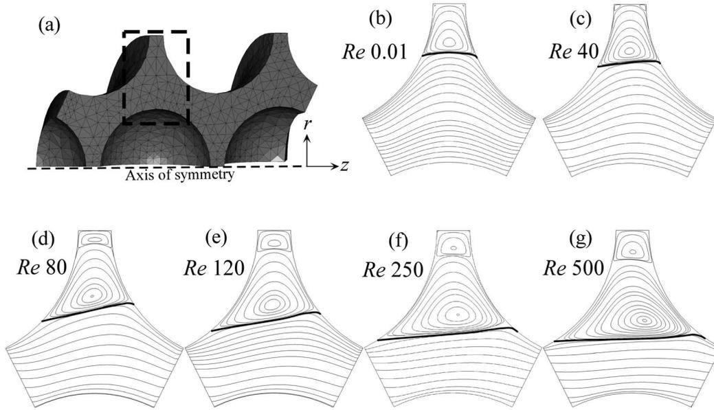
**Figure 1.** (a) 3-D rendition of 1/4th of the axis symmetric pores formed due staggered pattern of spheres. (b) Flow field shows a pair of corner eddies and a larger stationary eddy in the Darcy flow regime. (c) to (g) growth in eddies as flow rates increases from  $Re$  0.01 to  $Re$  500 to occupy a large part of the advective pore volume ( $n_e$ ). Bold black lines point at the separation between zones occupied by eddies and  $n_e$ . Thin black lines are streamlines.
