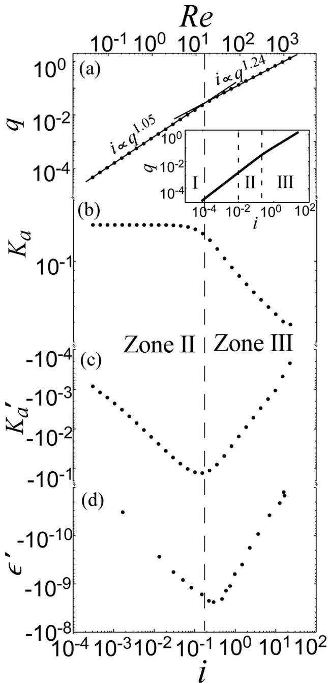
**Figure 4.** Characteristics of Forchheimer flow in Zone II and Zone III as shown by dependence of: (a) specific flux  $q$  [m/s], (b) apparent hydraulic conductivity  $K_a$  [m/s], (c) rate of change in apparent hydraulic conductivity  $K'_a$  [m/s], and (d) rate of change in eddy growth  $\epsilon'$  [-], on  $Re$  [-] and  $i$  [-].
