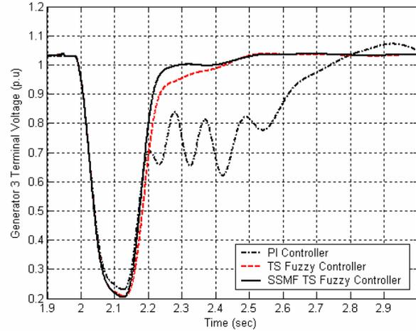
Fig 6. Generator 3 terminal voltage during the fault
