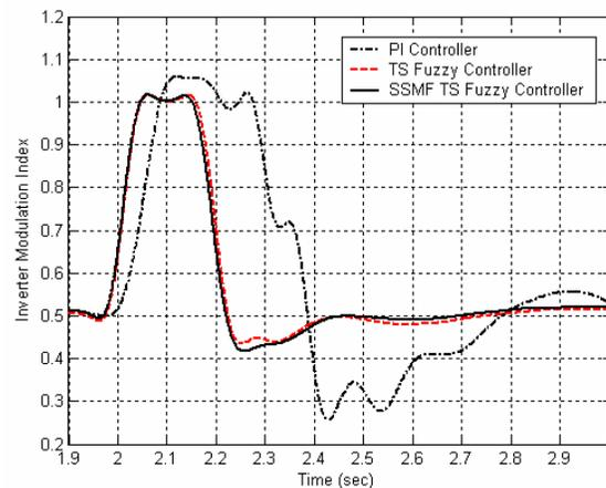
Fig 8. Inverter modulation index during the fault
