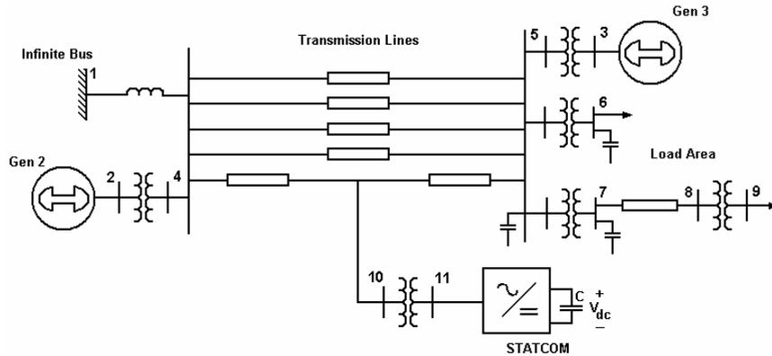
Fig 1. STATCOM in the multimachine system
